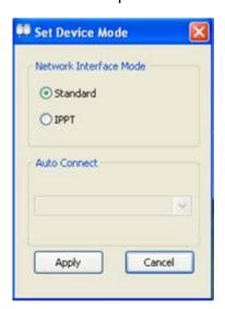
Select "Standard" and click "Apply." The device will reboot. This is identified by the momentary blinking of red on the device LED. VMBM can be used again to manage the device after the switch has completed successfully.
