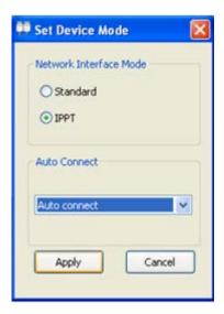
After making a selection for the Auto–Connect option, click "Apply." The device will reboot. This is identified by the momentary blinking of red on the device LED.
